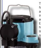
This pump is designed for continuous use and features a multiple switch option for automatic operation. Epoxy-coated cast iron housing is oil filled for lifetime lubrication and rapid heat dissipation.
