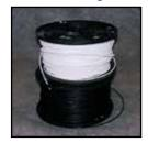
Raven Welding Rod is used for field seaming, repairs and detail work, such as installing pipe boots. Packaged in 10 lb spools, it is available in 4mm and 5mm sizes to fit most brands of extrusion guns. Raven Welding Rod is made from a thermally UV stabilized LLDPE resin and is available in both black and white to correspond with the color of geomembranes being utilized.
